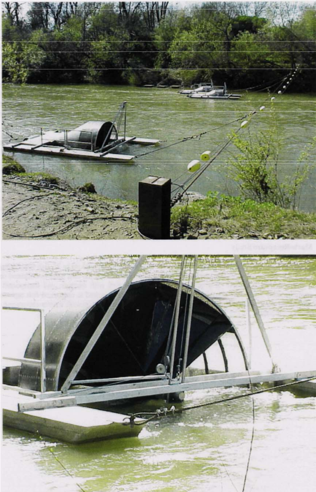
Figure 3-2. Rotary screw traps (under relatively high flow conditions) in the Russian River below the Inflatable Dam.
