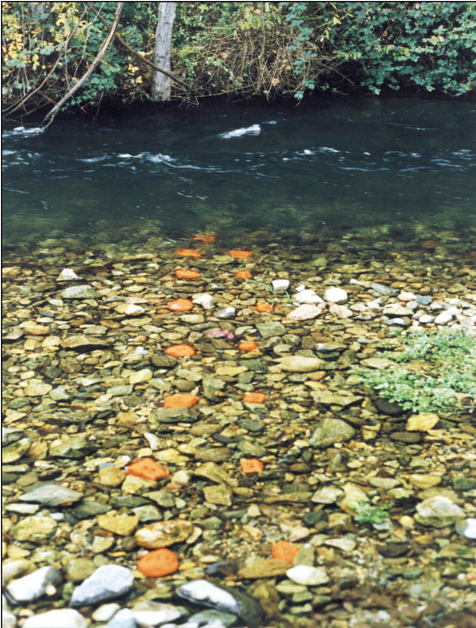
Figure 21. Photograph of typical tracer gravel placement along a cross section.
