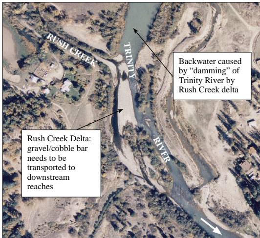
Air photo of Rush Creek Delta showing local sediment accumulation and upstream backwater "lake"
