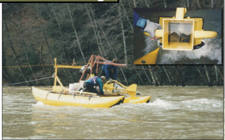
Sediment sampling during high flows measure the effectiveness of dam releases in routing gravel and sand through the river
