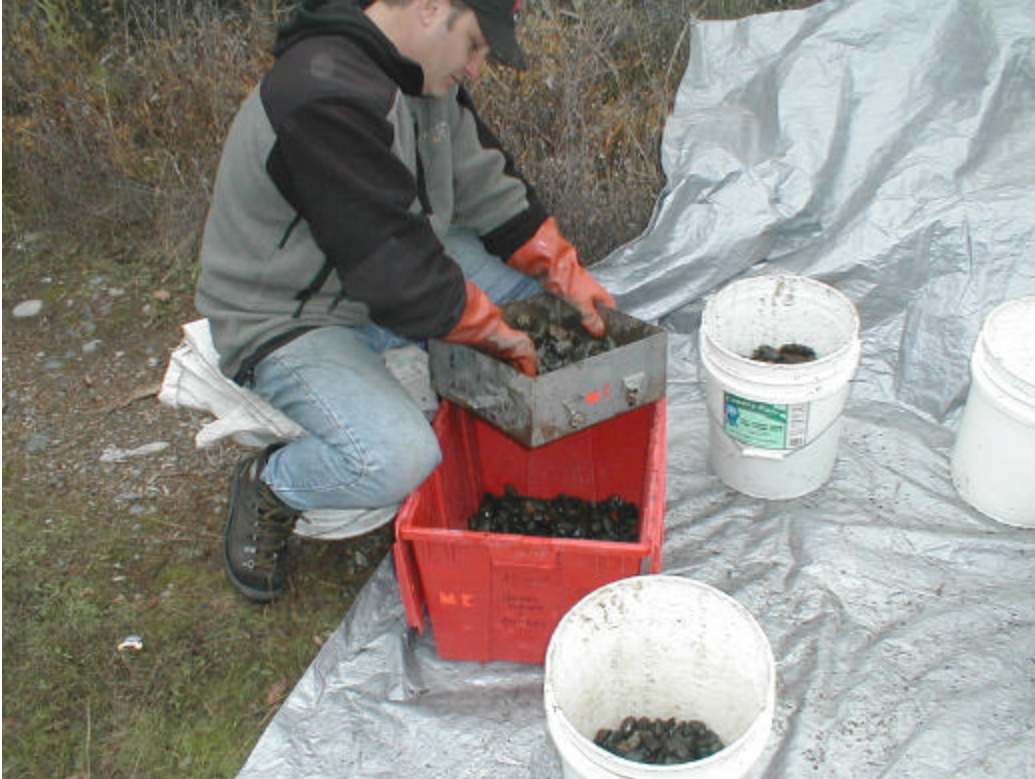
Figure 7. Initial wet sieving of bulk sample through 16 mm screen in rocker box.
