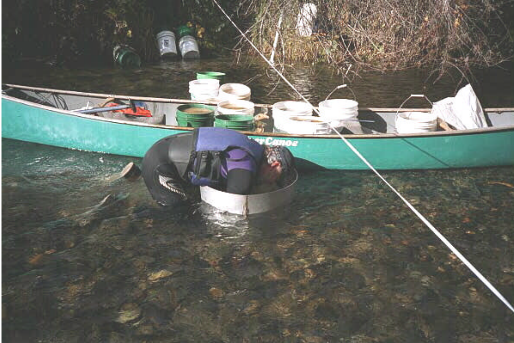
Figure 5. Bulk sampling using modified 2' diameter McNeil-type sampler. Canoe was used to retain buckets during sampling and transport to the bank for sieving.
