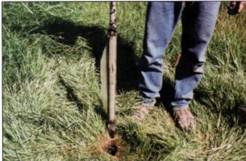
Figure 4. Method of soil-core collection from drained and undrained wetlands.
