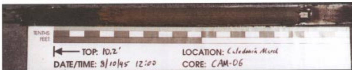
D. Deep soil layers (depth = 10.2–11.9 feet), showing transition from olive clay with hemic peat to gray clay.
