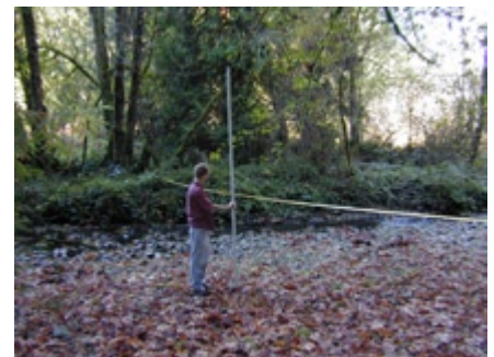
Salmon Forever cross-section at Graham Gulch. Comparison of cross-section data from year to year can reveal changes in sediment load and aggradation.
