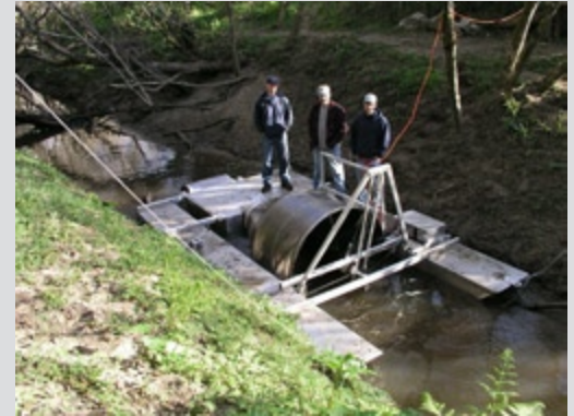
In 2003 Green Diamond and DFG, installed a motorized rotary screw trap and placed it in the channel about 2 miles from the mouth. The trap needs to be motor operated since even in spring the discharge can be too low to turn the trap. The motor driven screw trap, if successful, will allow an annual outmigrant population estimate of coho smolts for most of the Ryan Creek drainage.
