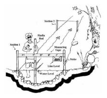
Note: Leave the string line attached to the stakes running across the stream. You will use this as a marker for the velocity measurement.
